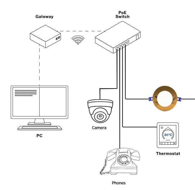
PoE lighting uses Power over Ethernet technology to connect, monitor, and control LED light fixtures used in smart building solutions. Smart PoE lighting reduces installation and operating costs by more than half and helps building owners meet wellness and sustainability goals. Since the low voltage PoE system does not require shielded cables, conduit runs are eliminated early in the construction process.
